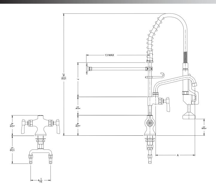
1-1/2" (29mm) hole for deck is recommended to accommodate 1/2" supply nipples.
