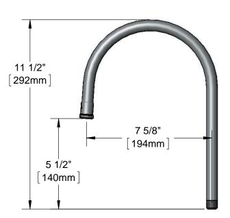
**Product Specifications:** Drawn Checked Approved Rigid Gooseneck w/ 7 5/8" Spread & Stream Regulator Outlet **KJG** JHB **DMH** Scale: Date: 1:4 10/04/13
