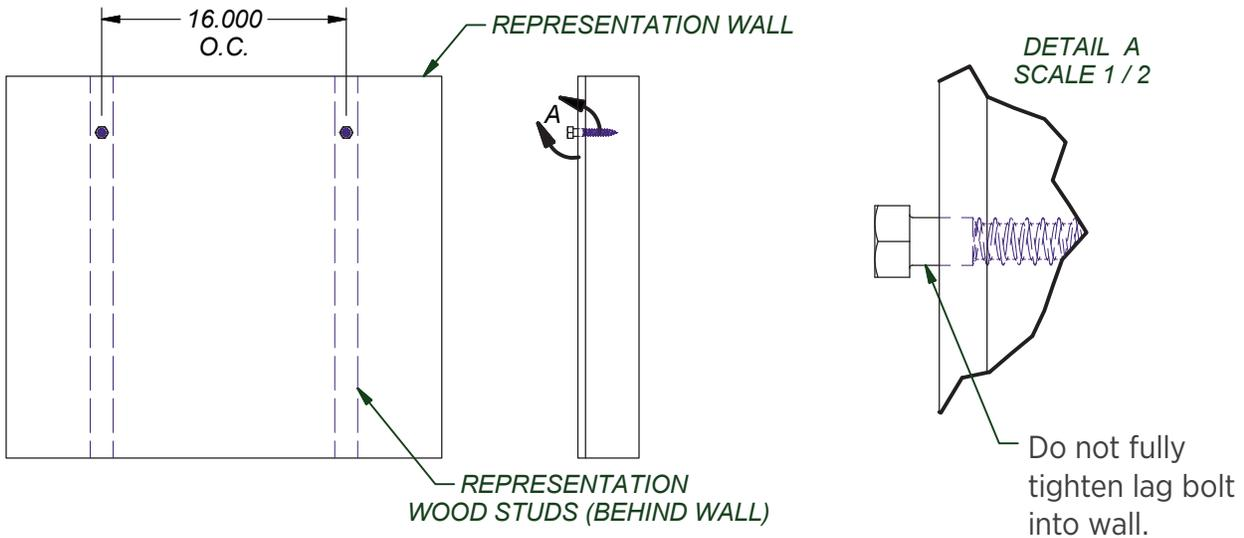
**STEP 1 - INSTALL LAG SCREWS (ITEM 1) INTO WALL
