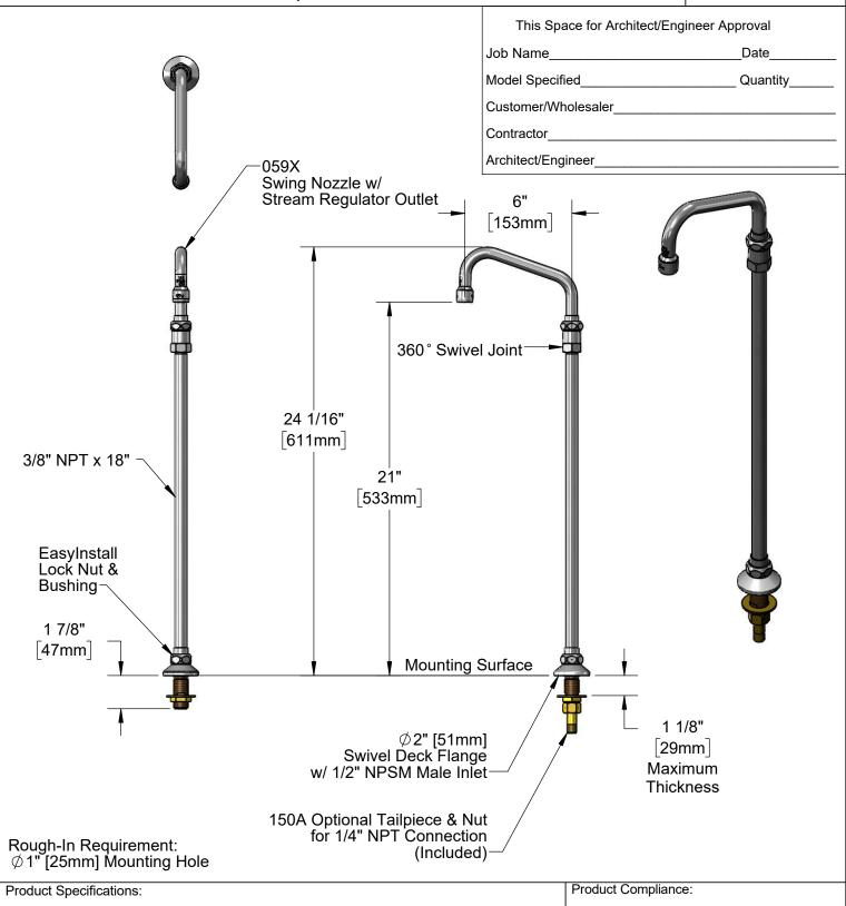
Swivel Deck Mount Dummy, 6" Swing Nozzle, Swivel Piece, Stream Regulator Outlet & 1/2" NPSM Male Inlet
