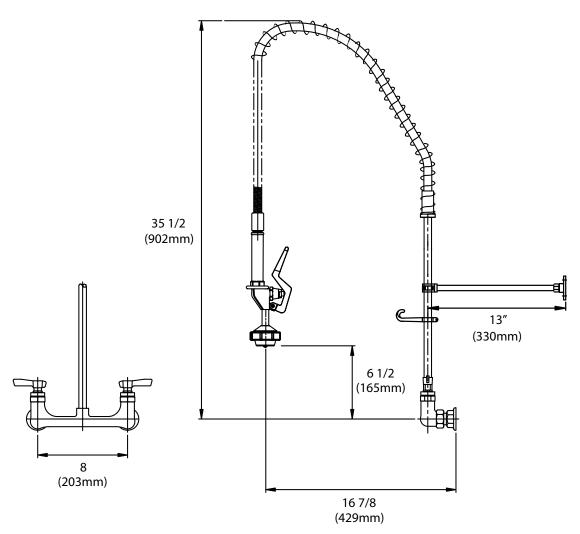
1-1/2" (29mm) holes for backsplash are recommended to accommodate 1/2" supply nipples. 1/2" NPT Female Inlets
