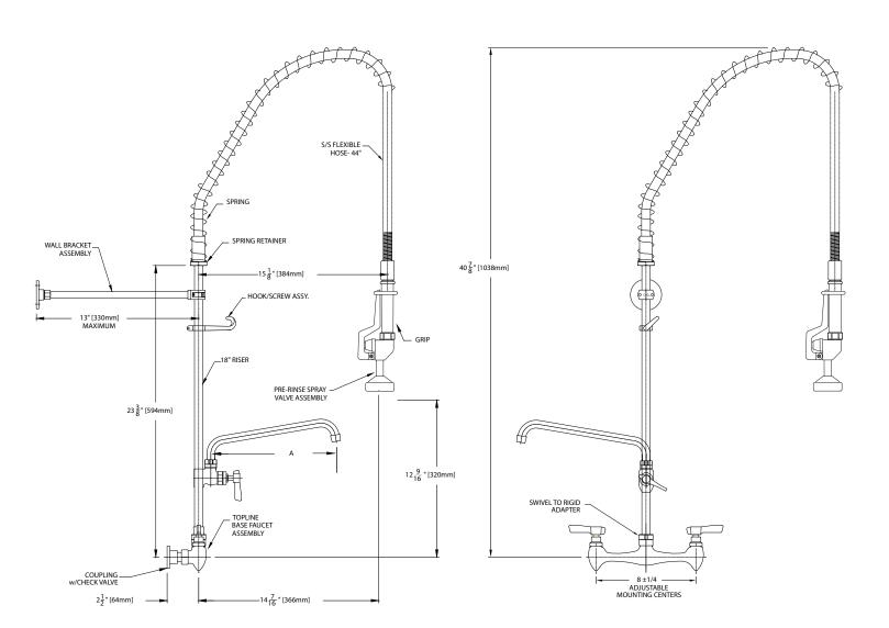
1-1/2" (29mm) holes for wall are recommended to accommodate 1/2" supply nipples.
