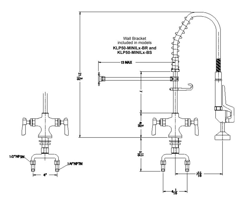
1-1/2" (29mm) hole for deck is recommended to accommodate 1/2" supply nipples.
