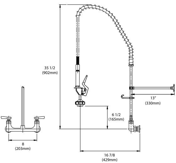
1-1/2" (29mm) holes for backsplash are recommended to accommodate 1/2" supply nipples.
